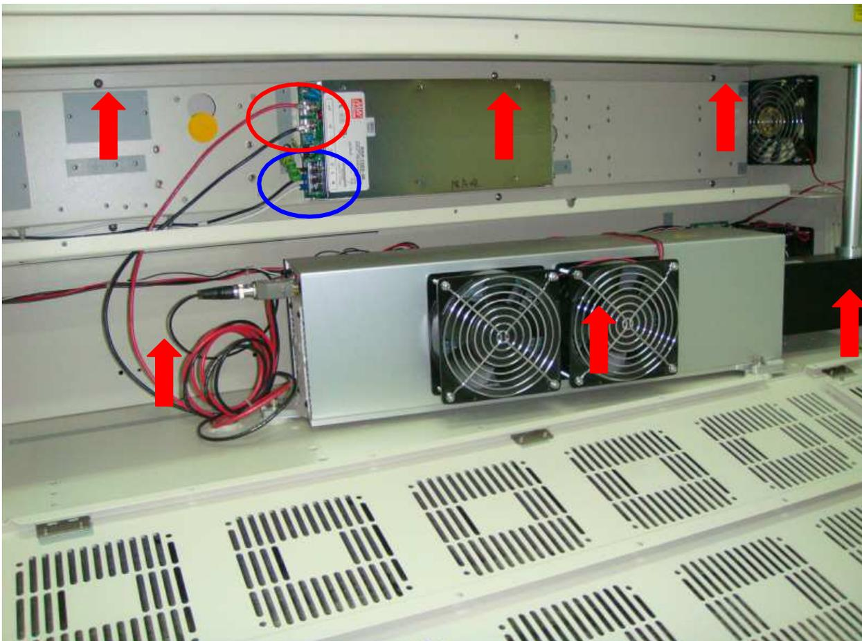
5. Dismount 3 screws on the power supply panel (see red circle below). The power supply can be changed to new one.
