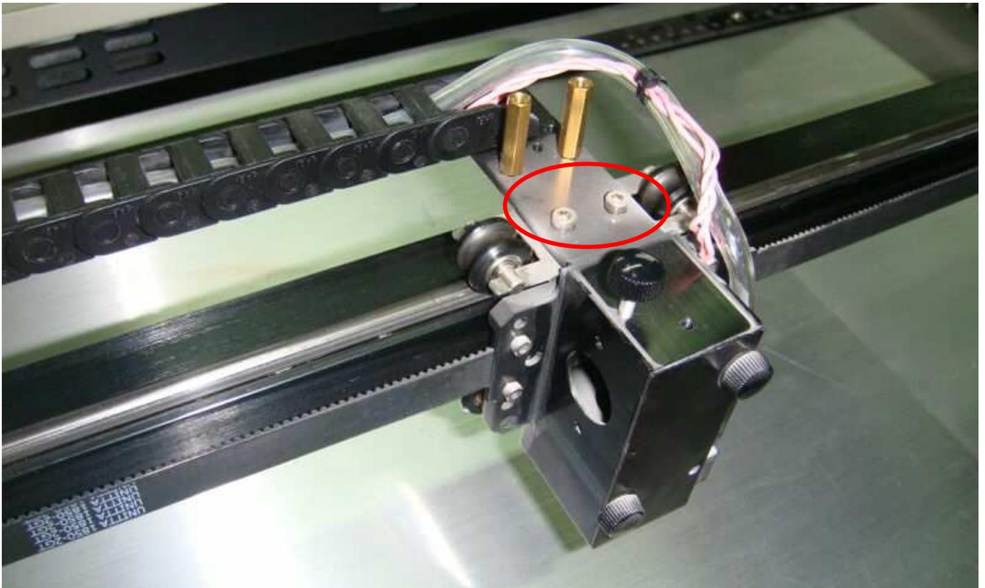
6. Unscrew the following screws to remove the A roller.
